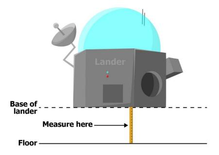
Size: When deployed/assembled, the lander must be at least 30 cm at its widest width.
